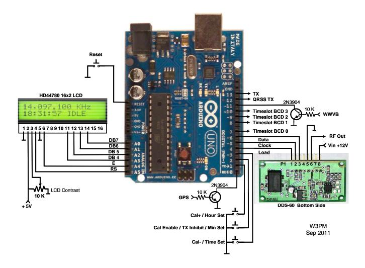
Arduino Uno / DDS-60 Schematic
